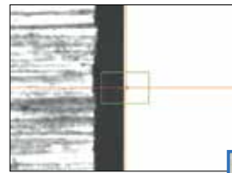
Edge Focus Tool This is a tool for focusing on a beveled edge.
