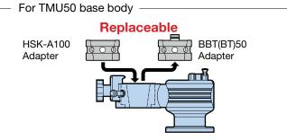
By replacing with another adapter (optional), different shank types become available as long as the base body is compatible with the adapter.
