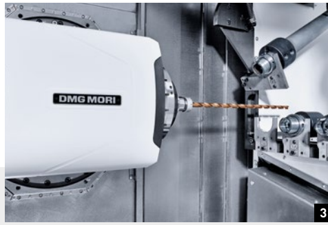
1: Tool chain magazine for up to 180 tools 2: Tool loading station with optimum accessibility from the front 3: Additional magazine for 6 oversized tools up to 700 mm length or ø200 mm (optional for all CTX gamma TC machines) 4: Disk magazine with 36 stations
