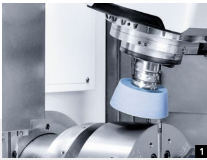
1: Acoustic emission sensor: Monitoring of the dressing process 2: Tool technology: Standardised grinding wheel holder with IKZ 3: In-process measurement: Measurement repeat accuracy up to 0.8–1.0 µm (Marposs Micromar 8)
