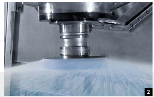
1: Acoustic emission sensor: Monitoring of the dressing process 2: Tool technology: Standardised grinding wheel holder with IKZ 3: In-process measurement: Measurement repeat accuracy up to 0.8–1.0 µm (Marposs Micromar 8)
