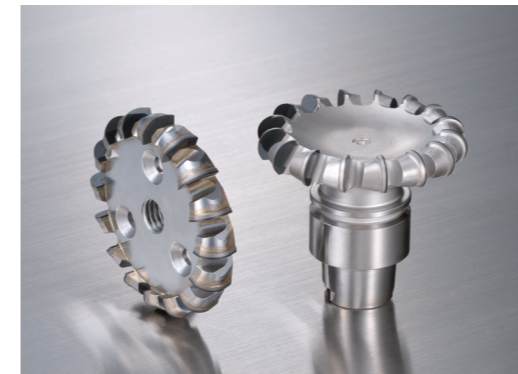
Tool Head Replacement Type Holder Integrated Type
