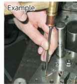
Punch driving with pins.
